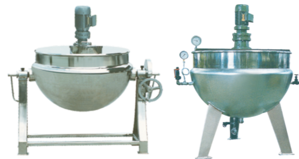
可倾式球形夹层锅 TILTING TYPE SPHERICAL SANDWICH POT 立式球形夹层锅
